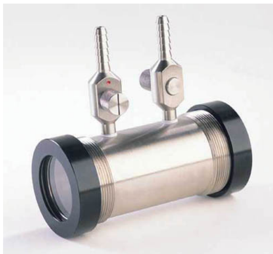
Figure 3.3: Gas cell. Gases are charged through one of the tubes on the side. The valves are closed when the partial pressure of the sample is adequate.
