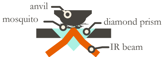
Figure 3.8: Diagram of an ATR crystal used to measure the IR spectrum of a mosquito.
